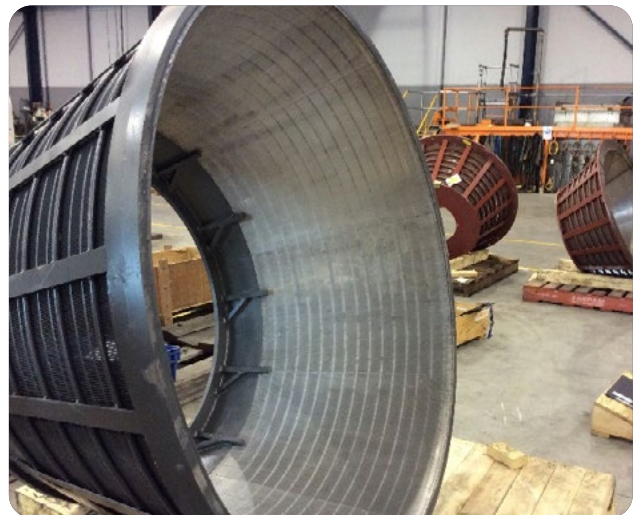
B. Coal Wash Buckets
