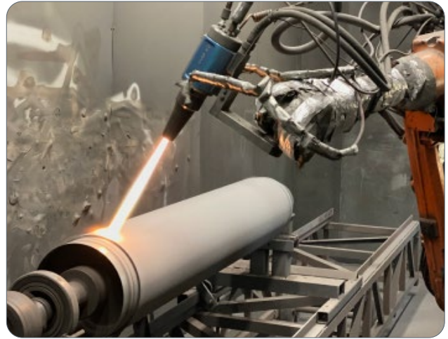
The HP HVOF coating a long shaft.
