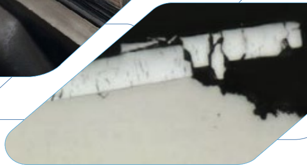
Figure 2: microscopic image of a failed Hardchrome coating after short service in an underground mine. Corrosive media penetrated through micro-cracks causing bi-metallic corrosion.
