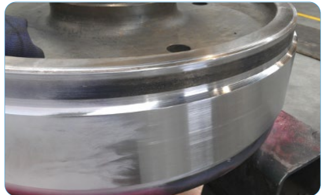
Damaged area is removed by machining built up with Laserbond® Cladding
