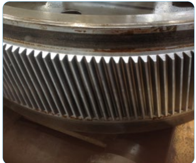
New gear teeth were cut as per the profile given the customer
