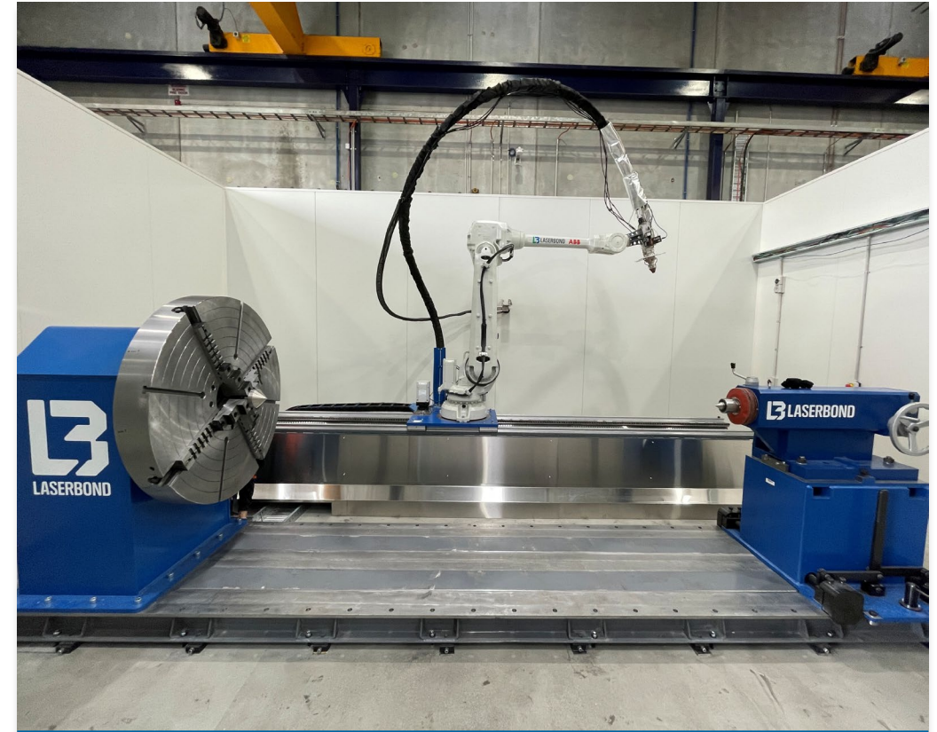
Laser cell in final factory testing
