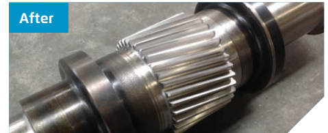
New gear teeth were cut as per the profile provided by the customer.
