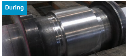
Damaged area is removed by machining and built up with LaserBond® Cladding.
