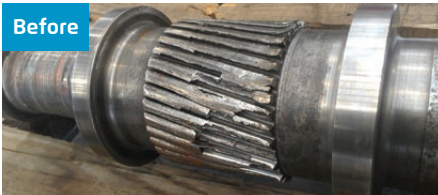
Damaged gear teeth of the mating gear.
